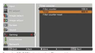
Press the SELECT button to select **Timer** and then use the Point ▲▼ buttons to set the timer. Select from (**Off/600H/900H/1200H/1500H/1800H/2000H**) depending on the use environment.
